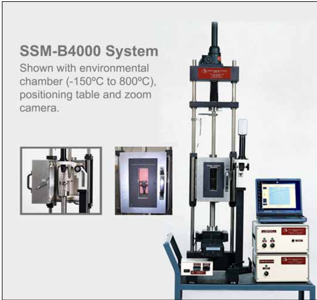
Fig. 5 The bench-top SSM system (Model SSM-B4000) is shown above with all optional accessories. ATC's patented SSM systems have been in use worldwide since 1991. In addition to performing the innovative ABI tests, the bench-top systems are also state-of-the-art universal testing machines with the SSM-Suite™ software icons shown below.
