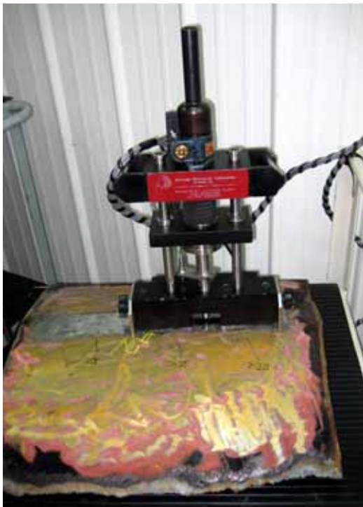
SSM-M1000 System testing a pipeline section
