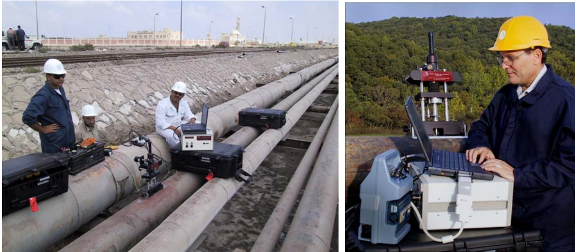
Fig. (1) Photographs of the SSM system used in testing 14-inch diameter pipelines: a Kerosene pipeline in Alexandria, Egypt (Left Photo) and a demo in Tennessee (Right Photo).
