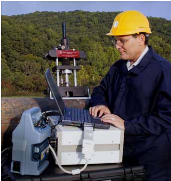
Fig. 1 Photograph of SSM system used in testing a 14-inch diameter pipeline.
