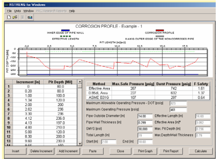
Fig. 9 The ABI-determined minimum ultimate strength was 54,800 psi, which meets Grade "A". Hence, the SMYS value of 30,000 psi for Grade "A" was used here to calculate a maximum safe operating pressure of 107 psi. Again, this is very close to the current operating pipeline pressure of 100 psi.
