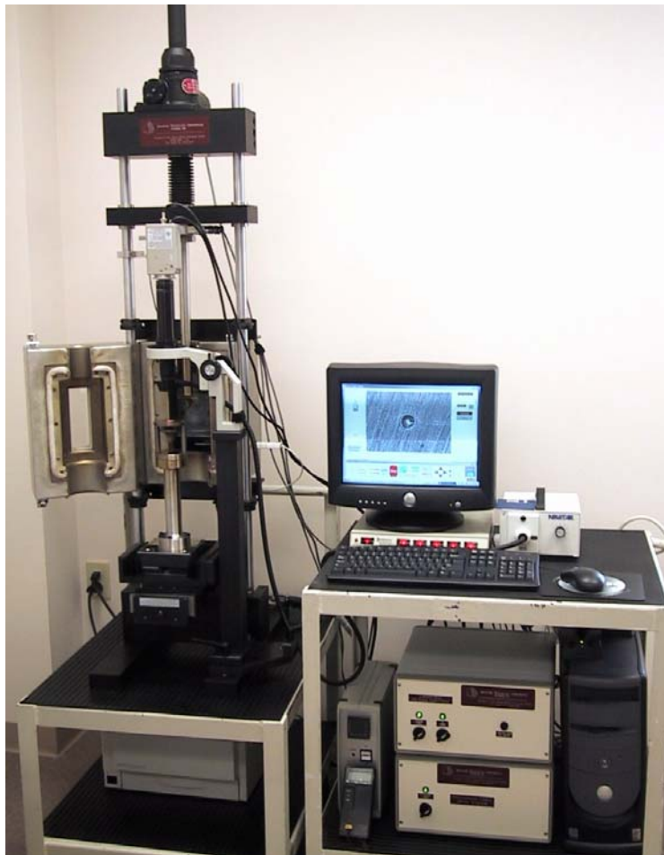
Fig. 1 The laboratory version of the Stress-Strain Microprobe™ (SSM) system is equipped with an environmental chamber for testing samples at low and high temperatures and a positioning table to allow accurate testing of specific weld areas and their heat-affected-zones.
