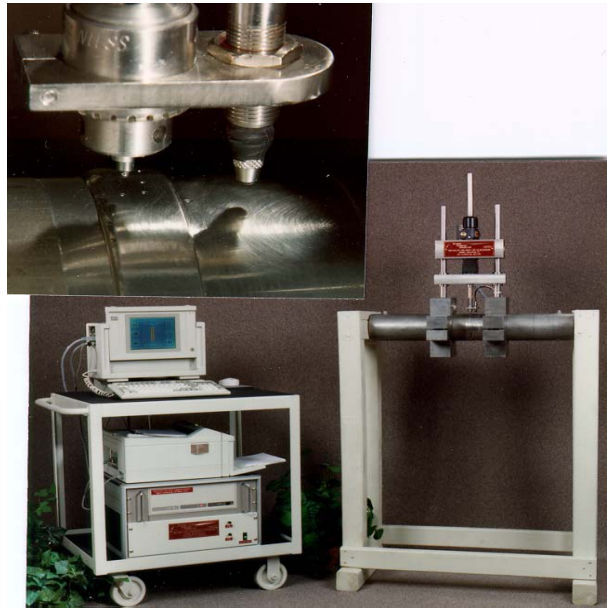
FIG. 1--A portable Stress-Strain Microprobe (SSM) system is used here for in situ testing of circumferentially welded type 347 stainless steel pipe (100 mm outer diameter and 5 mm thick). The pipe is held in a wooden stand to demonstrate this field application of the SSM system. Four aluminum V-blocks were used to temporarily attach the testing head (two column load frame) of the microprobe system to the pipe, allowing a 360° inspection of the stress-strain curve gradients in the weld and its HAZ. The inset photo is an enlargement of the 100 mm pipe, chuck (20 mm diameter) holding a 1.57 mm spherical tip indenter, and a displacement transducer mounted in a horizontal bracket. (The bench-top system, which is not shown here, has a support platen for laboratory specimen testing.)
