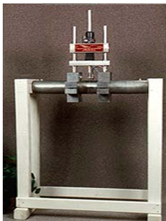
Figure 2a SSM on a 347 Stainless Steel Pipe
